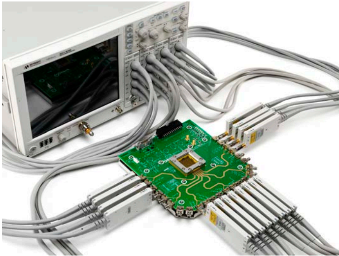
2- to 16-channel TDR/TDT/S-parameter measurement system.
