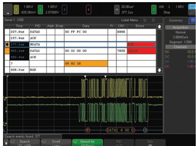
Figure 21. USB 2.0 trigger, decode and "lister" display.
