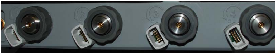
Figure 3 V-Series oscilloscope probe connectors
