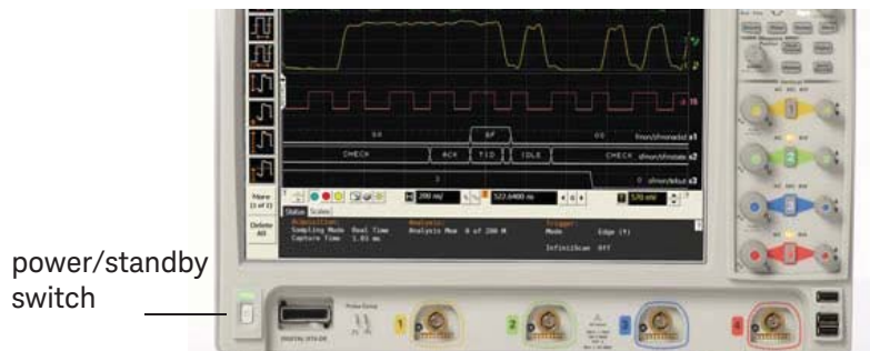
Figure 5 Turning On the oscilloscope
