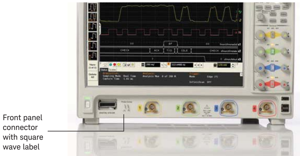
Figure 6 Verifying basic oscilloscope operation
