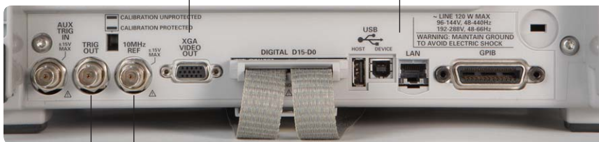
Built-in 10-MHz reference in/out port lets you synchronize multiple measurement instruments in a system.
