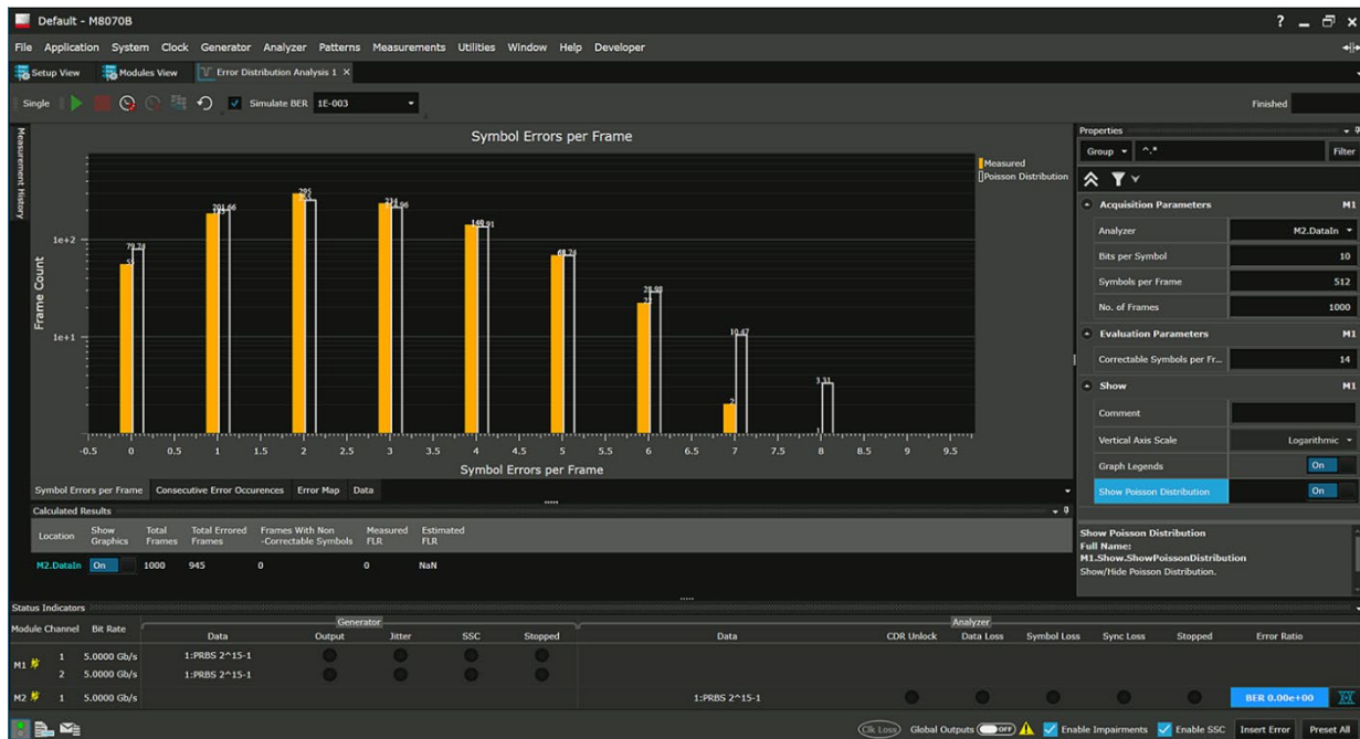
Figure 10. The error distribution analysis M8070EDAB provides multiple views to debug the error distribution. The figure shows an example of symbol errors per frame based on captured pattern streams, with the measured frame loss ratio, based on user-definable number of bits per symbol, correctable symbols per frame and frame length. Automated Receiver Calibration and Characterization for IEEE 802.3bs, OIF CEI-56G-VSR, PCI Express 5.0, CCIX, SAS and TBT 3 Interfaces
