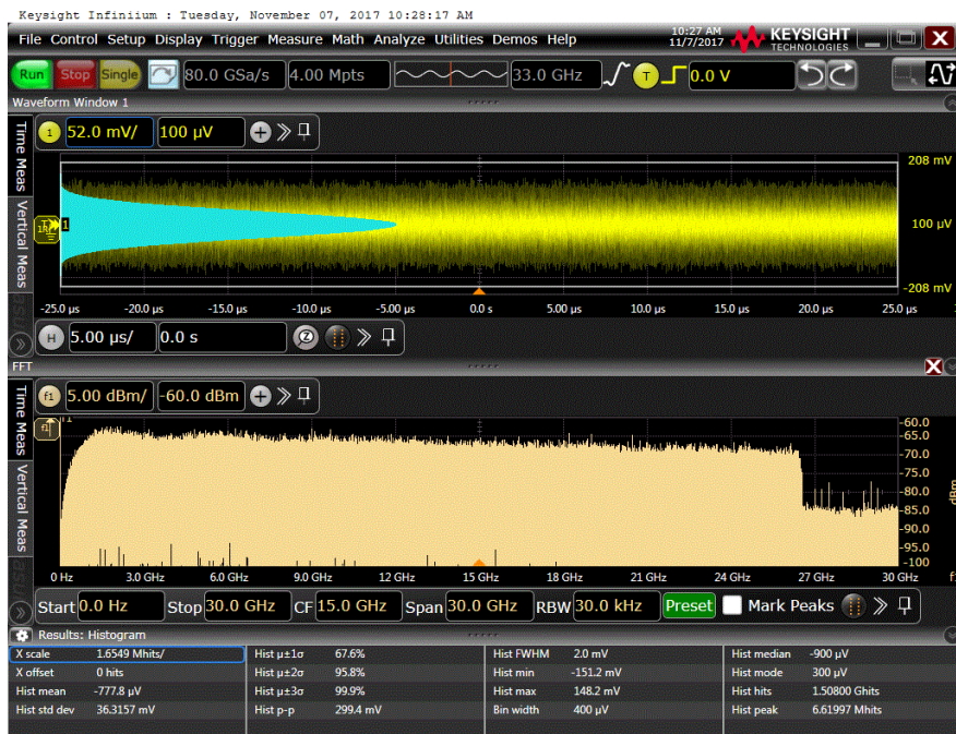
Figure 2: Random (gaussian) interference signal with a flat spectrum and bandwidth of 26 GHz, which corresponds to half of Nyquist frequency at 53 Gbaud symbol rate.
