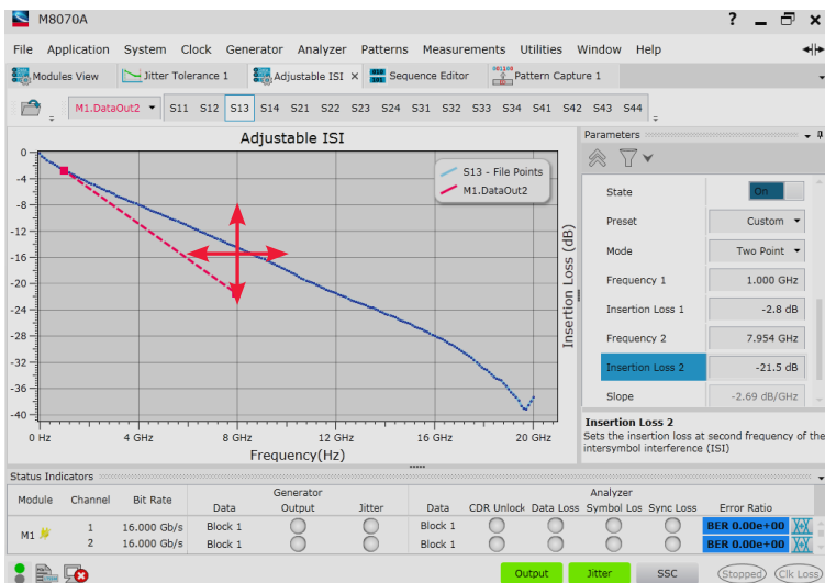
Figure 8. J-BERT M8020A offers integrated and adjustable ISI to emulate channel loss. ISI can be controlled for each channel independently via a graphical user interface. Frequency and loss points can be set. S-parameter files can be imported. The example shows a loss curve in blue for the imported S21 parameters for the 12.8 " trace of M8048A. The red line shows the loss parameter entry for M8020A.
