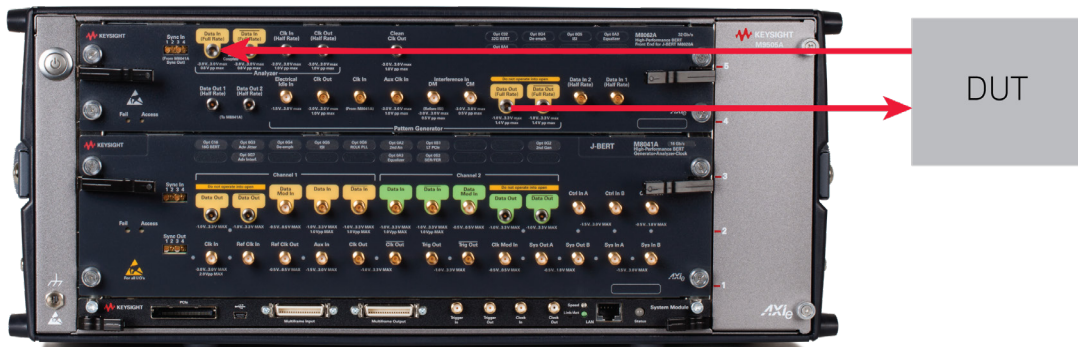
Figure 9. The J-BERT M8020A can be configured as a complete 32 Gb/s BERT for accurate receiver characterization. The M8062A 32Gb/s front-end provides a pattern generator with de-emphasis and ISI injection and analyzer CDR and CTLE.
