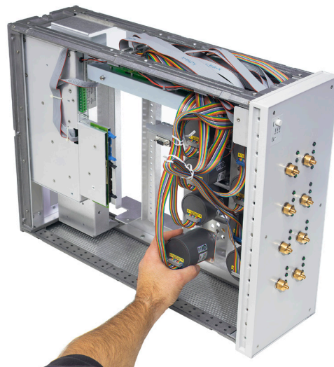
Figure 5: Easy to service the unit without disturbing the RF cabling
