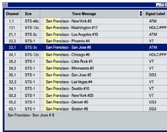
Figure 2: Clear tabular display of J1 or J2 path trace messages, or those identified based on a sub-string search.
