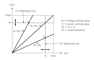
Figure 7-5. Output Characteristics
