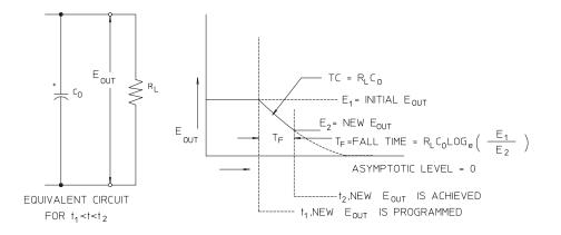
Figure 7-8. Speed of Response - Programming Down
