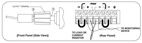
Figure A-2 Front/Rear Panel Terminal Connections
