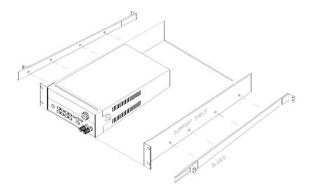
To install two instruments in a sliding support shelf, order support shelf 5063-9255, and slide kit 1494-0015.
