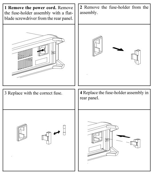
Verify that the correct line voltage is selected and the power-line fuse is good.
