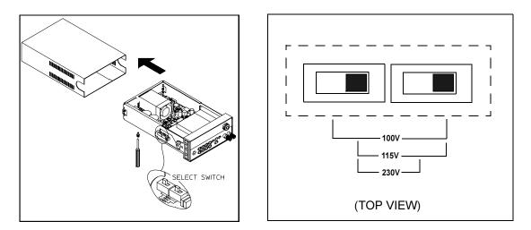
Figure 1-1. Line Voltage Selector (set for 115Vac)
