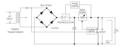
Figure 7-1. Diagram of Simple Series Power Supply
