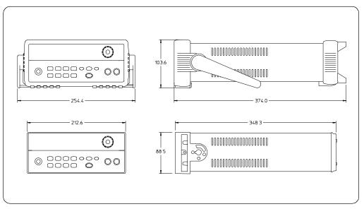
Figure 8-1. Dimensions of Agilent E3640A/41A/42A/43A/44A/45A Power Supply
