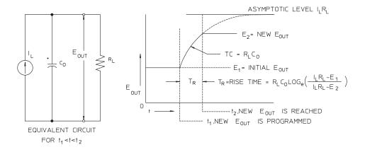
Figure 7-7. Speed of Response - Programming Up (Full Load)
