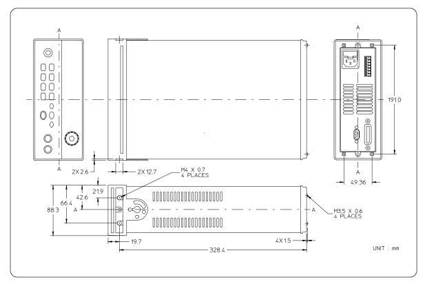
Figure 8-2. Dimensions for Rack mounting
