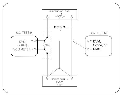
Figure A-1 Performance Verification Test Setup
