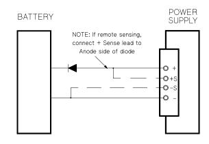
Figure 3-1. Recommended Protection Circuit for Battery Charging
