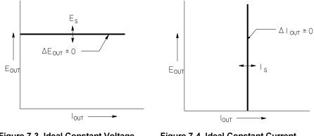
Figure 7-3. Ideal Constant Voltage Figure 7-4. Ideal Power Supply P
