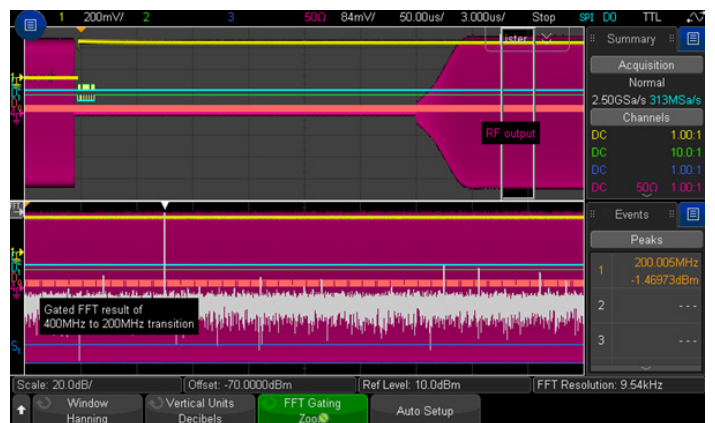
Figure 21d. RF signal settled down at 200 MHz as indicated in the search lister.
