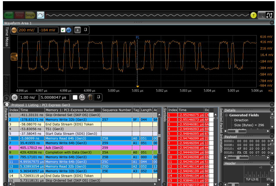
Z-Series decoding the PCI Express Gen3 packets.
