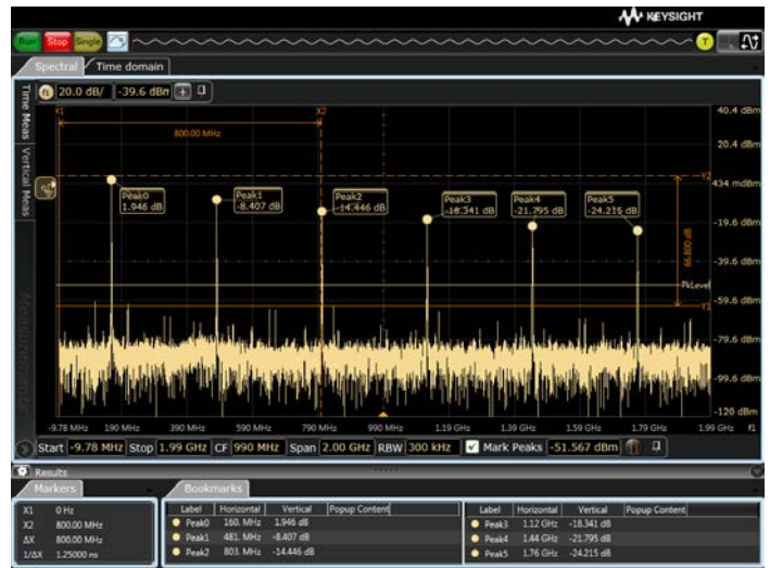
Peak readouts in the FFT plot.
