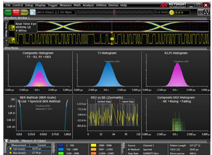
Multiple jitter analysis plots for enhanced visualization.
