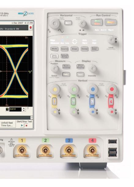
Starting with an **18-GHz**, **BNC-compatible connector**, an **ultra-low noise floor** front end design using **Faraday cage** technology ensures high signal integrity in its signal path.
