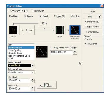
InfiniiScan software trigger setup screen
