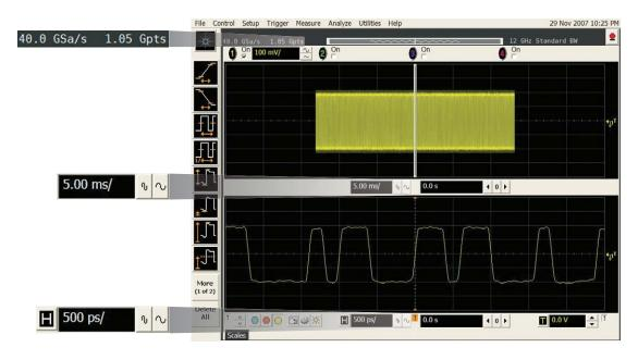
Acquiring 25 ms of PCI EXPRESS<sup>®</sup> Gen 2 data at 40 GS/s using 1 Gpts of memory will provide you the highest chance of capturing your signal of interest.
