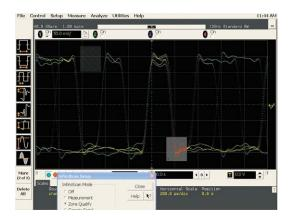
The "true" ease of use. Just draw boxes and the scope will trigger. The industry's only software event finder, "InfiniiScan Event Identification Tool" will provide the next level of ease-of-use for the scope triggering system.
