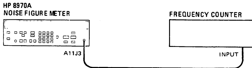
Figure 5-5. Second Converter LO Frequency Adjustment Setup
