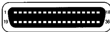
Figure 12b. HP 70611-60010 The standard I/O data cable is a five-foot cable with two female, 36-pin SCSI II type connectors.
