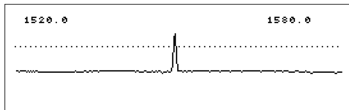
PRBS modulation graph showing raised noise floor.
