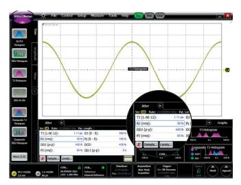
Jitter measurement showing an RJ component of 38 fs, indicating the ultra-low residual jitter of the 86108B's integrated clock recovery and timebase.
