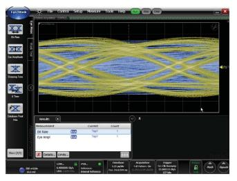
The Auxiliary clock recovery input makes it possible to analyze, and equalize, closed eyes.
