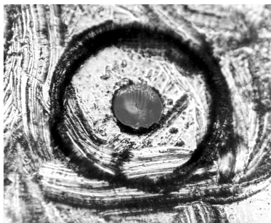
Figure 3-6. Damage from improper cleaning.
