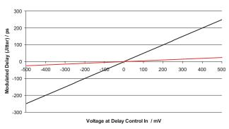
Figure 2: Modulated Delay (Jitter) vs Voltage Level at Delay-Control-Input for  $\pm 250 \text{ps}$  and  $\pm 25 \text{ps}$  settings
