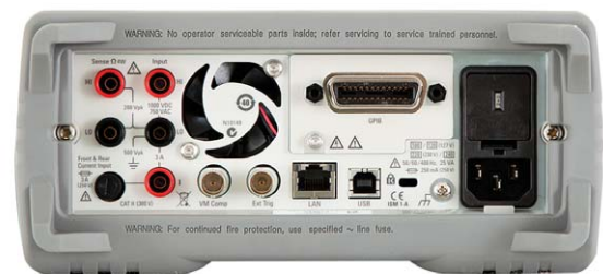
34461A DMM rear panel with GPIB option installed.
