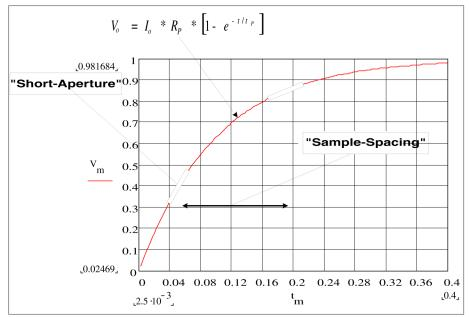
Capacitance is calculated by measuring the change in voltage ( $\Delta V$ ) that occurs over a "short aperture" time, ( $\Delta t$ ). This measurement is repeated at two different times during the exponential rise that occurs. An algorithm takes the data from these four points, and by linearizing that exponential rise over these "short apertures", accurately calculates the capacitance value.
