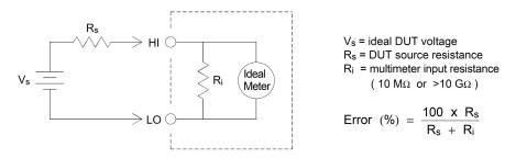
To reduce the effects of loading errors, and to minimize noise pickup, you can set the multimeter's input resistance to >10 G $\Omega$  (the HI–Z setting) for the 100 mVdc, 1 Vdc, and 10 Vdc ranges. The input resistance is maintained at 10 M $\Omega$  for the 100 Vdc and 1000 Vdc ranges.
