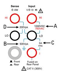
**Note:** The front-panel terminals are shown above. The rear-panel terminals are identical. The Front/Rear switch selects the terminal set to be used. *Do not operate this switch while signals are present on the front or rear terminals.* The current-protection fuse is on the rear panel.
