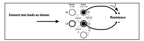
To null-out the test lead resistance:
