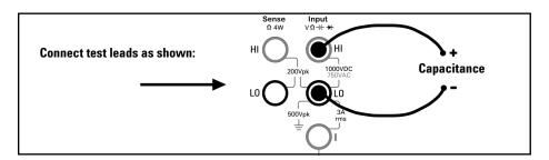
To null-out the test lead capacitance:
