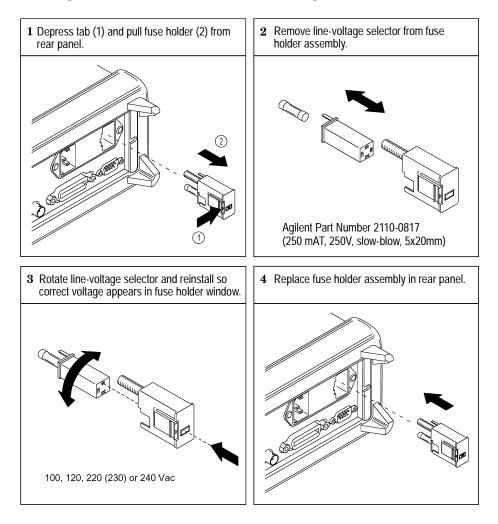
Verify that the correct line voltage is selected and the power-line fuse is good.
