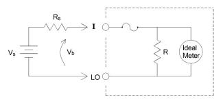
$V_s$  = source voltage  $R_s$  = DUT source resistance  $V_b$  = multimeter burden voltage R = multimeter current shunt
