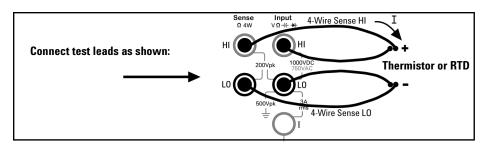
All 4-wire temperature measurements are made with auto-zero on.
