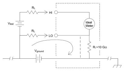
$R_L$  = lead resistance  $R_i$  = multimeter isolation resistance Vground = voltage drop on ground bus
