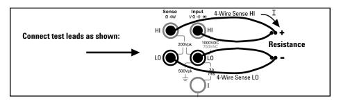
All 4-wire resistance measurements are made with auto-zero on.
