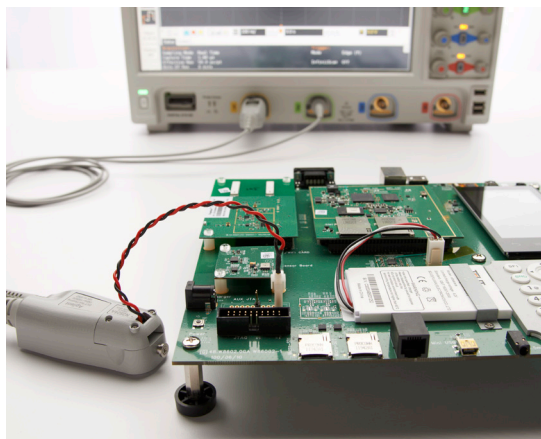
N2820A high-sensitivity 2-channel current probe
