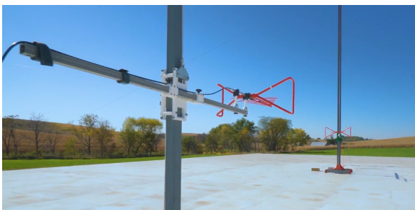
Figure 3. This CISPR antenna test was performed at our outdoor OATS on its CALTS-compliant ground plane.
