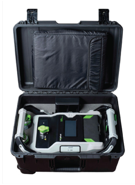
iPA shown with iAK-0600A ruggedized transport case with full PIM testing accessories
