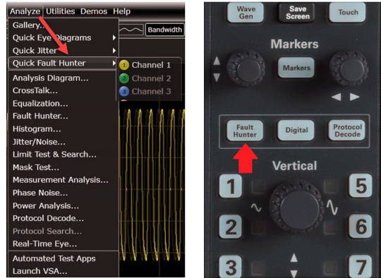
Figure 2. Using an EXR-Series oscilloscope, select Fault Hunter from the Analyze menu (at left) or use the front panel shortcut key (at right)
