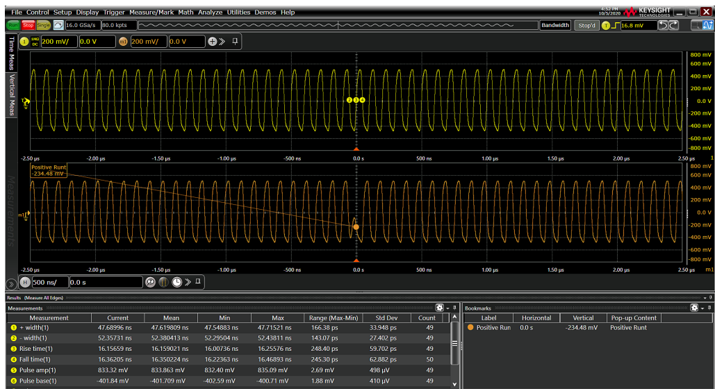
Figure 6. After clicking the view button, Fault Hunter will take you to the error it found
