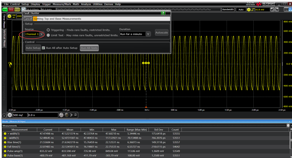
Figure 3. Any one channel can run Fault Hunter to produce a baseline of the mean and standard deviation of common measurements
