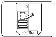
Turn the battery selector switch to LR6.
