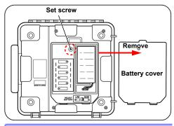
Connect the battery pack to the instrument. (Align the protrusions.)
