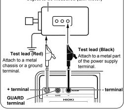
Clip the alligator clip at the end of each test lead to the object under test.
