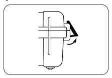
While raising the entire latch, place a finger on the top of the latch and pull it out.
