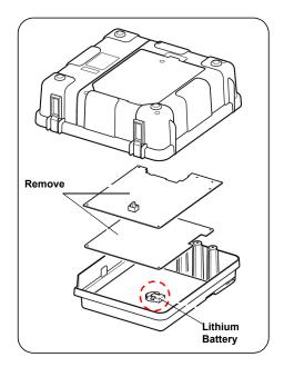
4. The battery is located on the remaining PCB as shown in the illustration on the previous page.
