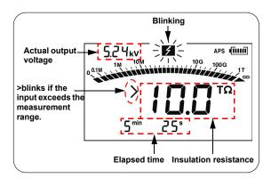
If > blinks, the input value is out of measurement range. Example: >  $10.0 \text{ T}\Omega$  means "larger than  $10.0 \text{ T}\Omega$ ."
