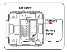
3. Place six LR6 alkaline batteries into the battery compartment. (Replace all six at the same time)
