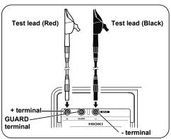
4. Clip the ends of the test leads to the circuit to be tested. When the voltage exceeds 50 V, the mark and keyler key lamp blink.
