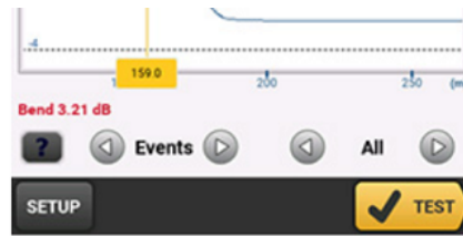
Bend as seen on an OTDR trace
