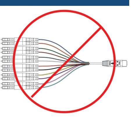
The MPO connector on both the Optical Power Meter and Light Source eliminates the use of costly and complicated fan-out cords to test MPO fiber trunks.
