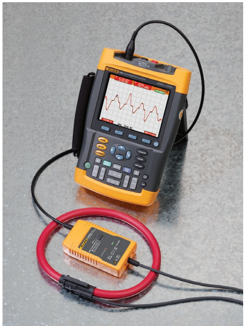
i6000s connected to a Fluke 199C ScopeMeter.
