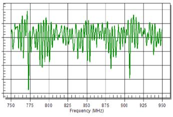
Figure 1. Typical Return Loss Sweep
