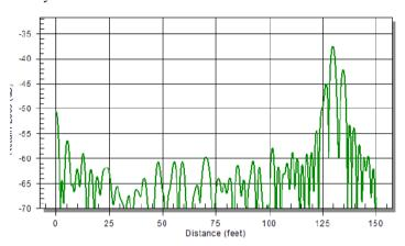
Figure 3. Typical Distance-to-Fault Loss Sweep
