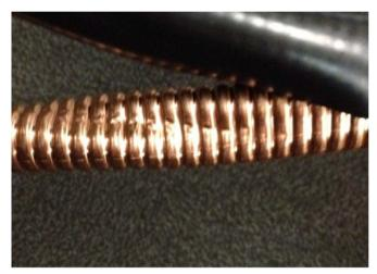
Figure 9. Cable Damage
