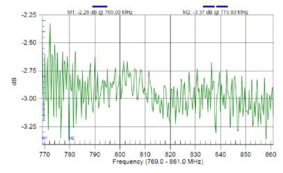
Figure 2. Typical Insertion Loss Sweep
