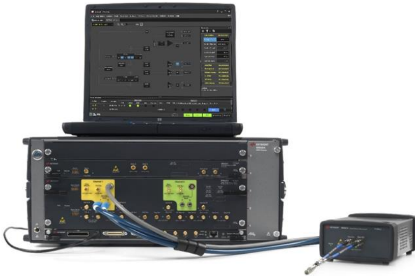
Figure 32: M8040A BERT system with M8045A PG, M8046A ED, and M8057A remote head
