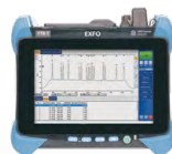
Optical Spectrum Analyser FTBx-5235
