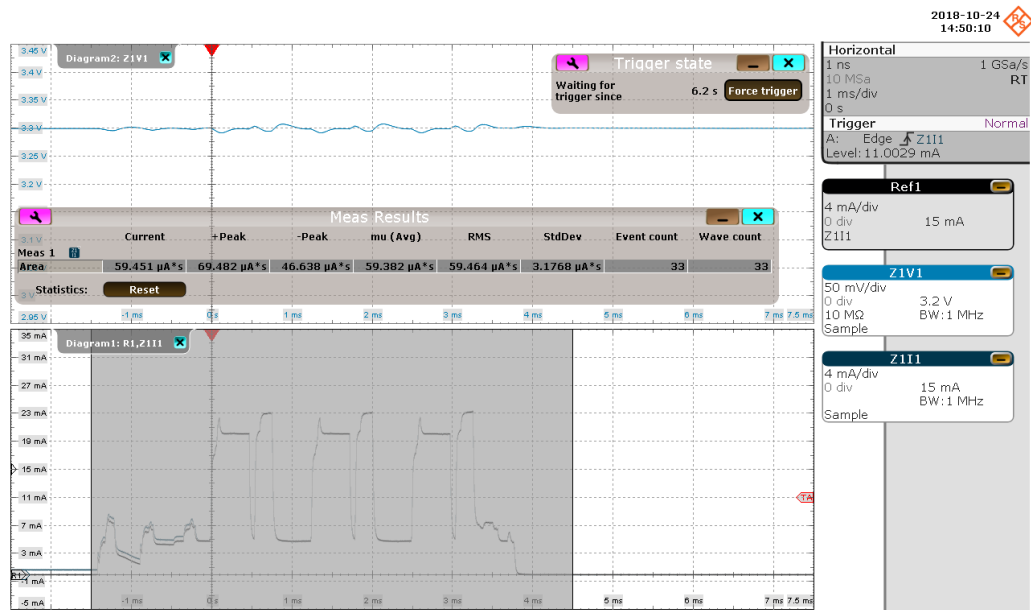
Figure 11 Bluetooth advertising event with only marginal capacitance present. The current waveform is also stored as a reference waveform.
