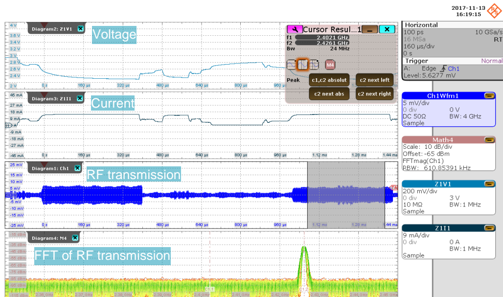
Figure 20 Gated spectrum measurement of Bluetooth frequency and hopping evaluated with near field probe The two consecutive transmissions differ in frequency of 24 MHz (top: 2.4021 GHz, bottom: 2.4261 GHz).
