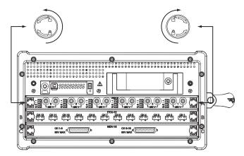
**4** Grasp the two knobs and slide the input module out of the recorder.
