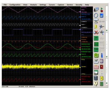
• **Scope mode** - Scope mode acts like a digital storage oscilloscope, providing high time-base resolution for viewing high-frequency signals. Scope mode is useful for timing and synchronization analysis, transient capture, and high-speed testing. It
