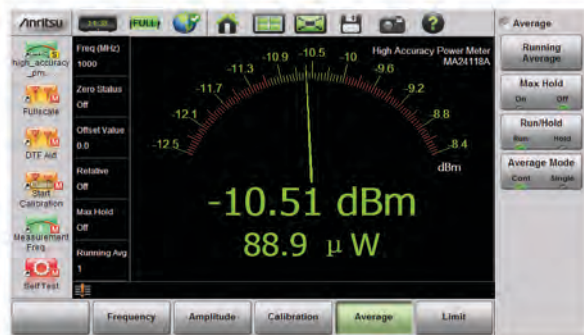
Power Level Within Limits (Green Text and Needle)
