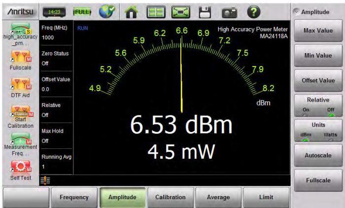
Figure 9-3. Autoscale to Zoom In on a Measurement
