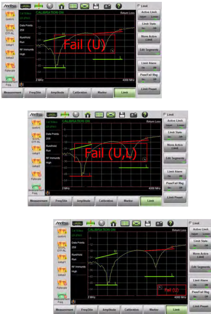
Figure 3-22. Pass/Fail Message Turned On
