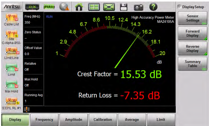
Figure 9-14. Measurement Value Beyond Reverse Limits Indicated by Red Text
