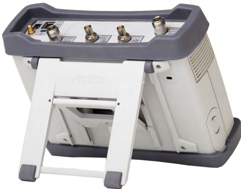
Figure 1-2. Tilt Bail Extended (different model shown)
