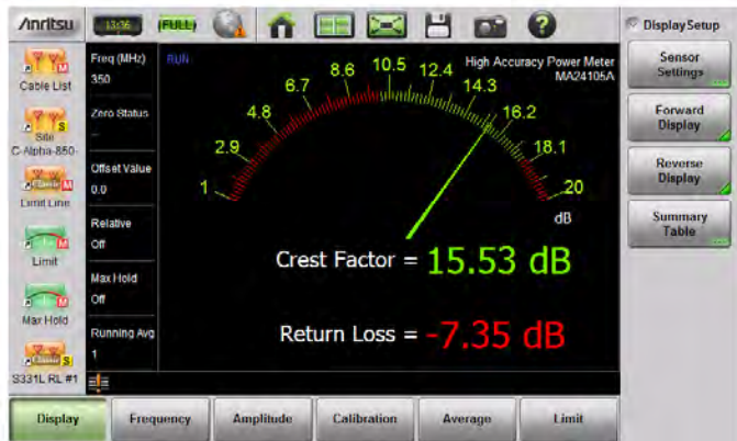
Figure 9-11. Forward and Reverse Measurement Combinations
