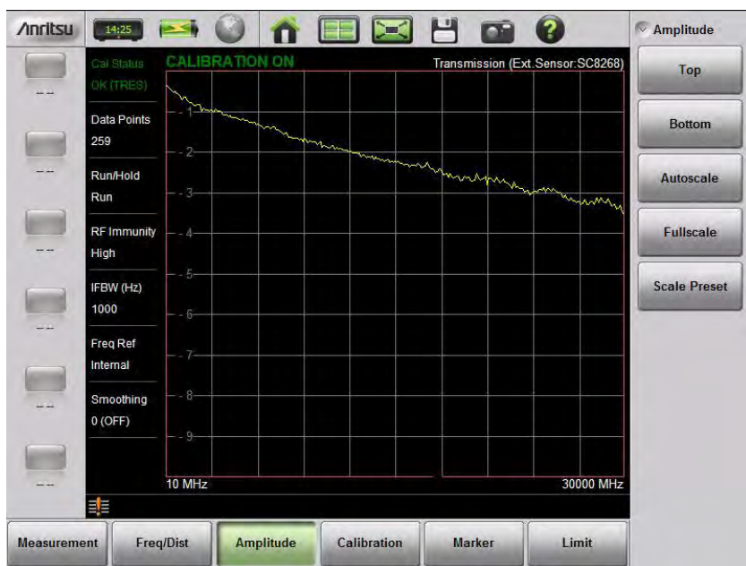
Figure 3-15. External Sensor Transmission Measurement Example
