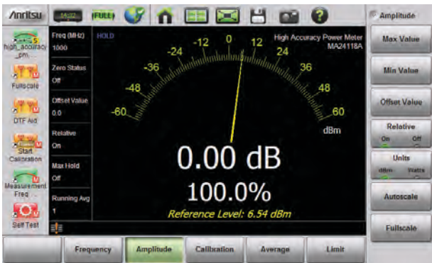
First Power Level, Relative On
