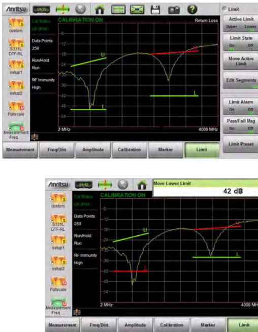
Figure 3-21. Moving Limit Line Segments
