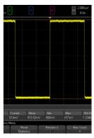
Another averaging mode. However, instead of waveform-to-waveform averaging, this performs point-to-point averaging. This allows you to capture glitches and aperiodic signals while still reducing some of the random noise riding on the signal.
