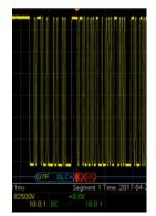
A unique mode that is used specifically to capture pulses, rare events, or infrequent glitches. Memory is wasted when you capture the downtime between infrequent events in the normal acquisition mode. With segmented memory, you're able to cut that time out and focus on the portions of the signal you want to analyze with even more detail.
