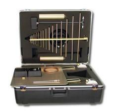
Frequency Range:20 Hz - 2 GHz Impedance:50  $\Omega$
