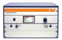
A front panel display indicates the operational status and fault conditions. All amplifier control functions, and status indications are available remotely using GPIB/IEEE-488, RS-232, fiber-optic serial, USB, or Ethernet. Interface connectors are located on the back panel. Local and remote operation is managed by a switch on the front panel.
