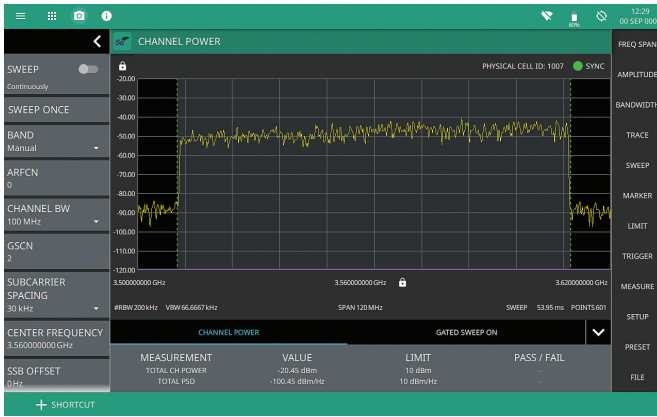
Field Master MS2080A Channel Power Measurement on 100 MHz 5G Bandwidth Carrier (Left) with Time Domain Gated Sweep Applied (Gate Set Up Shown Right)
