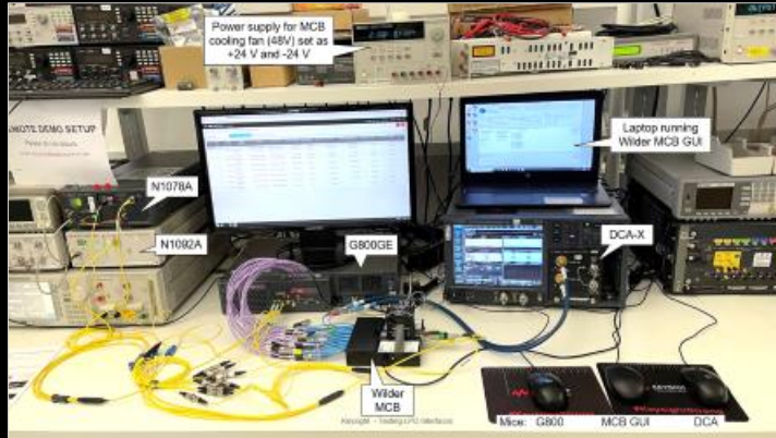
LPO setup in Keysight's lab
