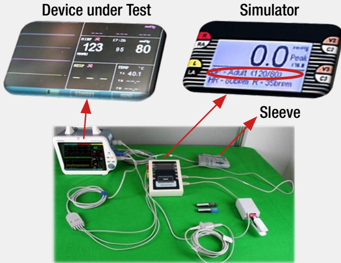
Figure 33: Complete set-up for testing non-invasive blood pressure monitors
