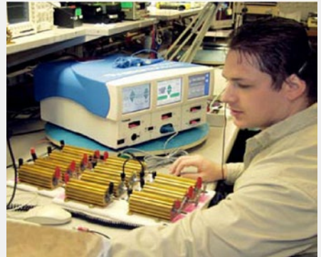
Figure 64: Test setup for testing HF surgical equipment with the SECULIFE ES PRO
