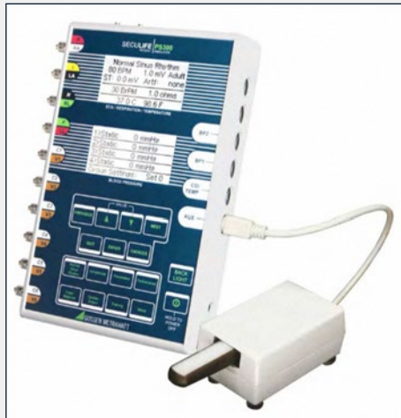
Figure 43: Connecting an SpO 2 module to the SECULIFE PS300 patient simulator
