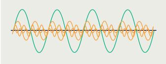
Multiples of basic oscillation. Possibly resulting in overheating of equipment and malfunctioning of circuit breakers and fuses
