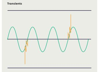
Extremely brief overvoltages which can reach several thousand volts. Possibly resulting in destroyed power supply units and IT hardware damages
