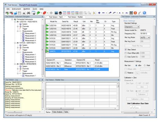
Figure 5. Multi-list display format of Keysight N1918A power analysis manager supports more than 20 USB power sensors simultaneously
