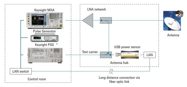
Figure 1. Typical test setup for continuous monitoring of the received power at a satellite antenna tower
