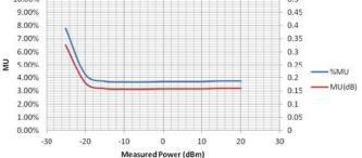
Figure 3. Long term drift performance of U8480 Series USB thermocouple power sensors and its impact to measurement uncertainty over power range
