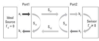
Figure 7. S-parameter correction
