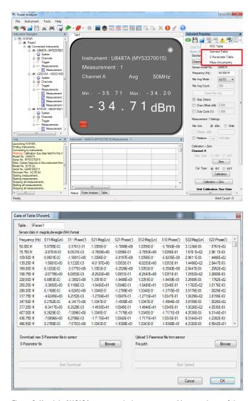
Figure 8. Keysight N1918A power analysis manager enables easy input of the DUT gamma and S-parameter files into the sensor's memory for gamma and S-parameter corrections
