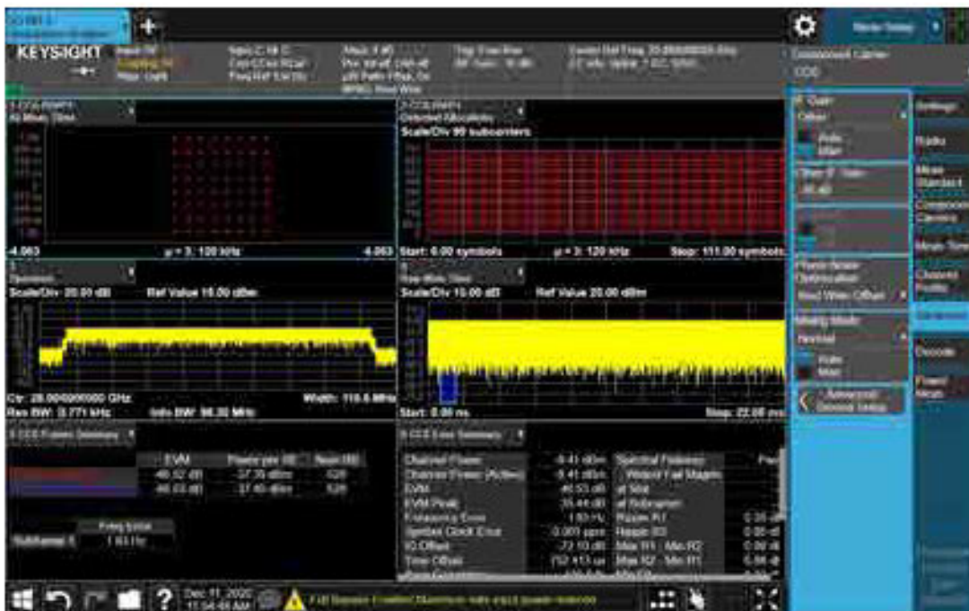
Figure 3. Configurable windows allow you to quickly characterize this 5G 28 GHz 1CC signal
