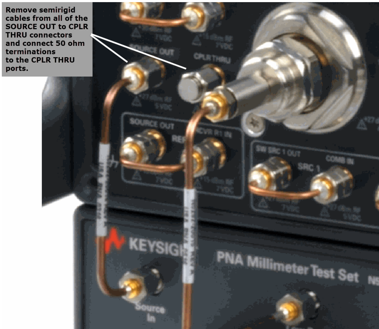
Figure 3-7 Remove Semirigid Cables and Connect 50 termination (1250-4261 (3.5 mm) or 0955-2394 (2.4 mm)) to the CPLR THRU Ports
