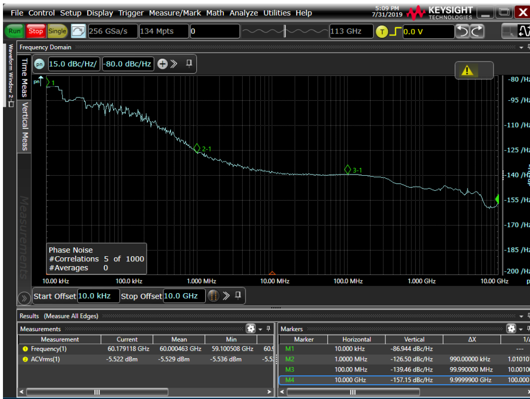
Figure 6. UXR phase noise measurements
