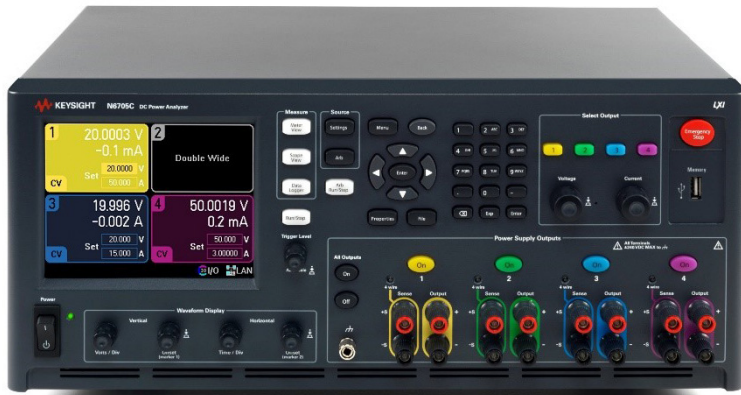
Figure 2. Keysight N6705C DC power analyzer provides five instrument functions in a single instrument – power supply, voltmeter / ammeter, oscilloscope, arbitrary waveform generator, and data logger
